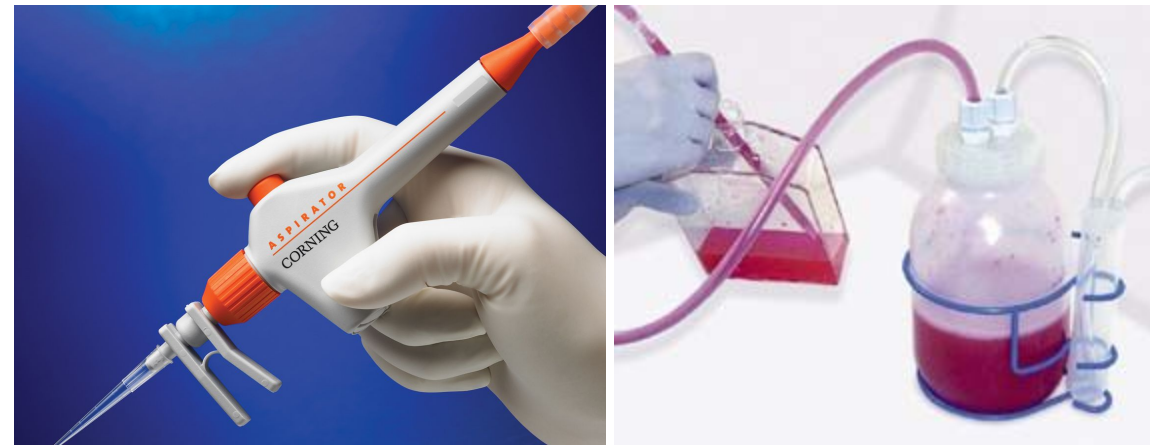
Figure 2. A typical aspirating pipette and waste reservoir for aspirating liquid during adherent cell feeding.
